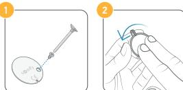
Remove the screw and then the cover of your key fob, and replace the battery (1x 3 V Lithium Panasonic or Energizer CR2032).
