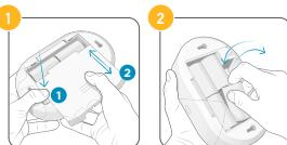
Remove the back cover and replace the batteries (4x 1.5 V alkaline D).
