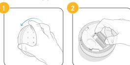
Open the keypad and replace the batteries (2x 1.5 V alkaline AA).
